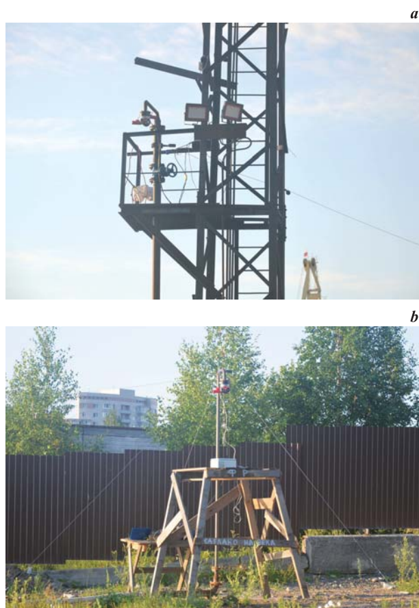
Fig. 3. Location of the RFM of type FR-LSD-S10Ub-IR at a height of 7.5 m ( a ) and 3.2 m ( b ) during testing
