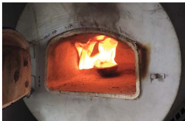
Fig. 13. The outburst when heating polyurethane
