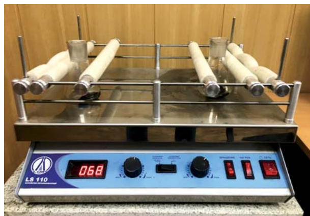
Fig. 4. Shaking the crushed sample with the residues of the combustion initiator
