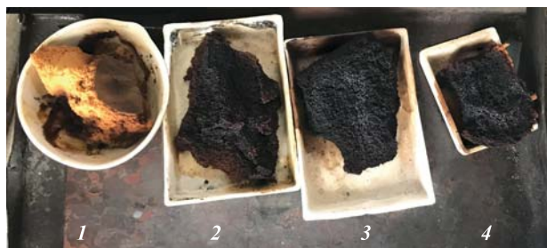
Fig. 3. Charred at t = 200\text{ }^{\circ}\text{C} polyurethane samples: 1 — 5 min; 2 — 10 min; 3 — 15 min; 4 — 20 min
