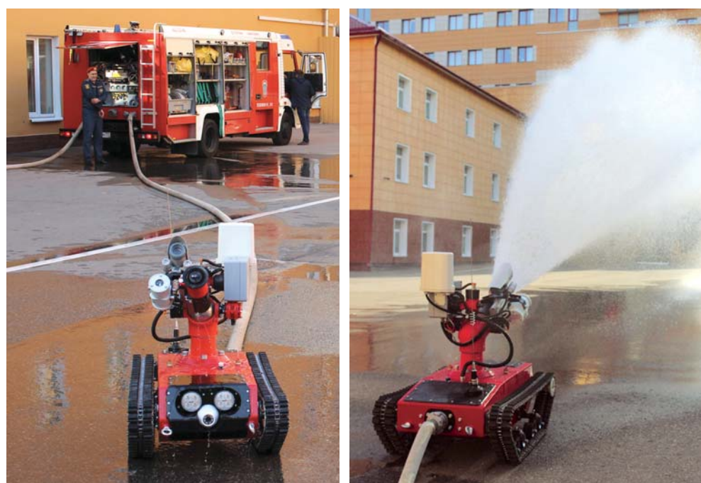
Fig. 4. Mobile robotic fire suppression unit
