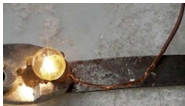
Fig. 3. Air gap that is equal to the thickness of the wire insulation and prevents the occurrence of a short circuit in the automobile electrical system
